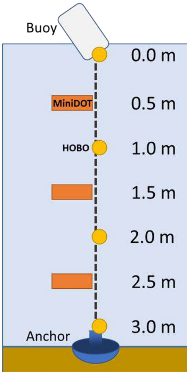
FIGURE 2. Example of a datalogging buoy, though instrumentation and depths vary. In West Hill Pond, the buoy was anchored at 20 m depth, and had five miniDOTs at 2m, 7m, 10m, 14m, and 18m deep.
